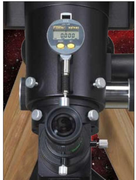
**ONE ACCESSORY** astroimagers especially like is the Fine Focus Indicator, a digital micrometer with resolutions of 1 micron or 10 microns. You can also display focus position on a computer with optional interface cables. ASTRONOMY: WILLIAM ZUBACK
