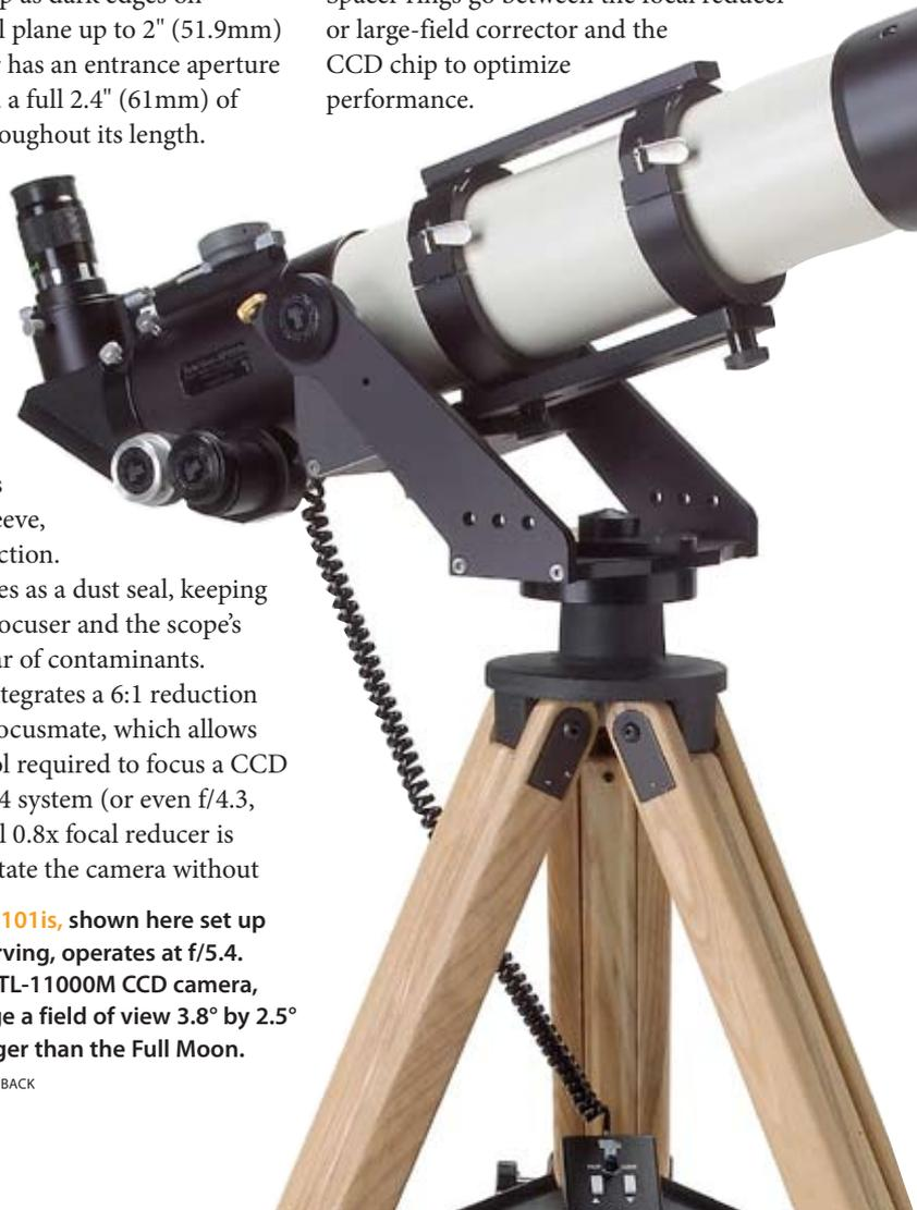
**TELE VUE'S NP101is**, shown here set up for visual observing, operates at f/5.4. Attach SBIG's STL-11000M CCD camera, and you'll image a field of view 3.8° by 2.5° — 38 times larger than the Full Moon.
