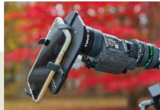
▲ Adding to the adaptability of the system is a simple setup for capturing images seen in the night-vision monocular with a smartphone. Using a method explained in the text, the author made all the accompanying astronomical images with his Apple iPhone 6s pictured here.
