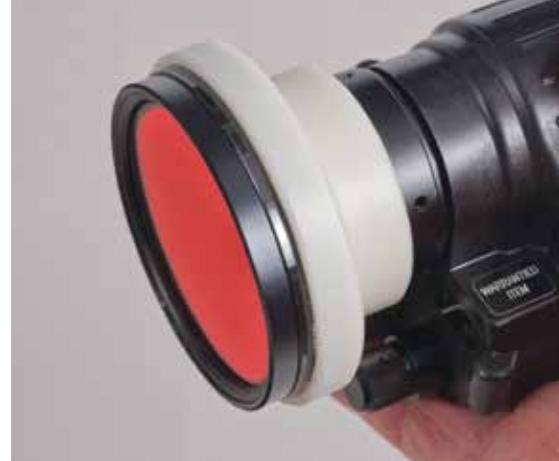
▲ After Tele Vue's Al Nagler treated the author to views of faint hydrogen-emission nebulae with a filter-equipped monocular (described in the text), the author made this plastic piece on a lathe to fit a 3-nm hydrogen-alpha filter over the objective of the monocular he tested. The setup was used for the pictures of Cygnus and Orion on the facing page.
