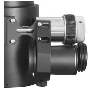
Installed Focusmate Driver shown from below to illustrate finished assembly (front of the scope is facing down). Notice the contact between the Drive Wheel and the fine focus knob on the Focusmate. Also, the Drive Wheel is off-center of the motor so that when the motor is rotated, the Drive Wheel disengages from the Focusmate.
