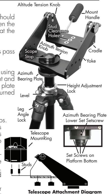
**WARNING:** Rotating the Tele-Pod head while the azimuth tension knob is tightened could cause the azimuth bearing to unscrew and separate.
