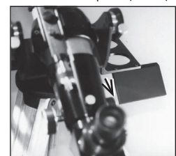
Typical DSC / Computer mounting plate on right Caddy. Note focuser knob clearance with plate (arrow).
