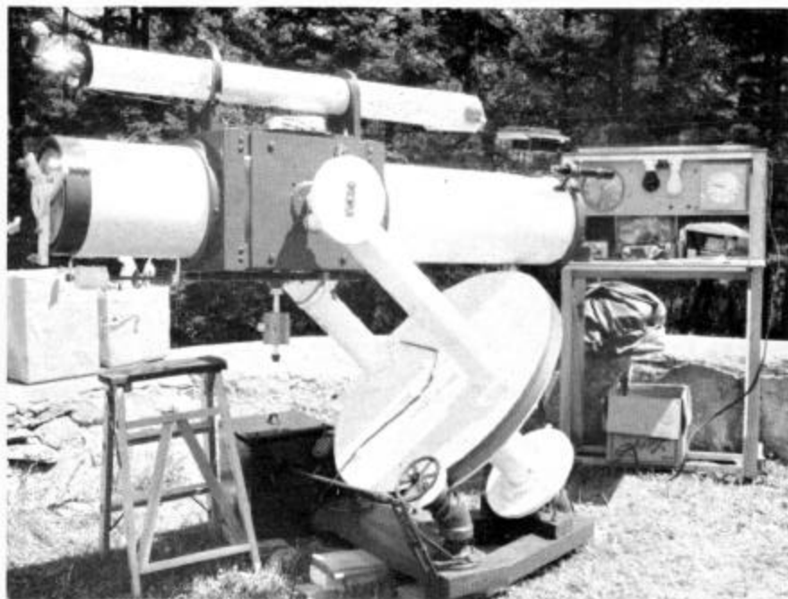
Berton C. Willard's 8-inch reflector won first prize. A counterweight beneath the main tube balances the long guiding telescope mounted on top. In the right background is the well-equipped control console. Stellafane photographs by Robert E. Cox.
