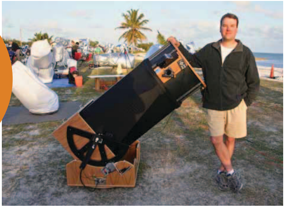
Mike Lockwood gets ready to observe through his 20-inch f/3 test Dobsonian reflector at the 2009 Winter Star Party held on West Summerland Key in Florida. He ground and polished the mirror, and Starmaster Portable Telescopes built everything else. Note how compact the telescope is, even sporting a 20-inch aperture. No ladder required here! Lockwood Custom Optics
