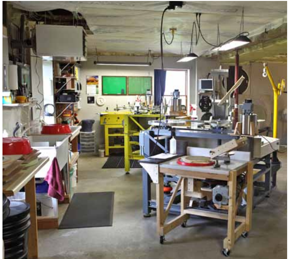
Lockwood Custom Optics , located near Philo, Illinois, currently has four mirror-grinding machines with mirror-figuring capacities of 14, 22, 34, and 60 inches. Lockwood Custom Optics
